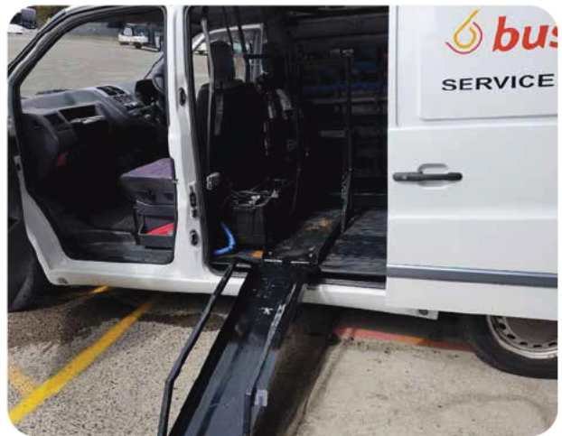
Spare wheels are safely unloaded on the near side of the repair vehicle away from the traffic flow
