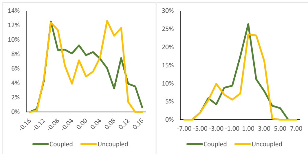
Figure 44 – PDFs of Lateral acceleration (left) and yaw rate (right) of unladen 5-axle dog at 40 km/h through the slalom
