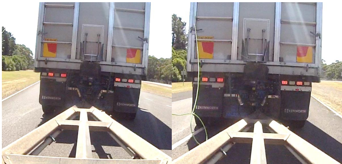
Figure 18 – Maximum lateral travel of the tow-eye with no coupling funnel relative to the coupling
