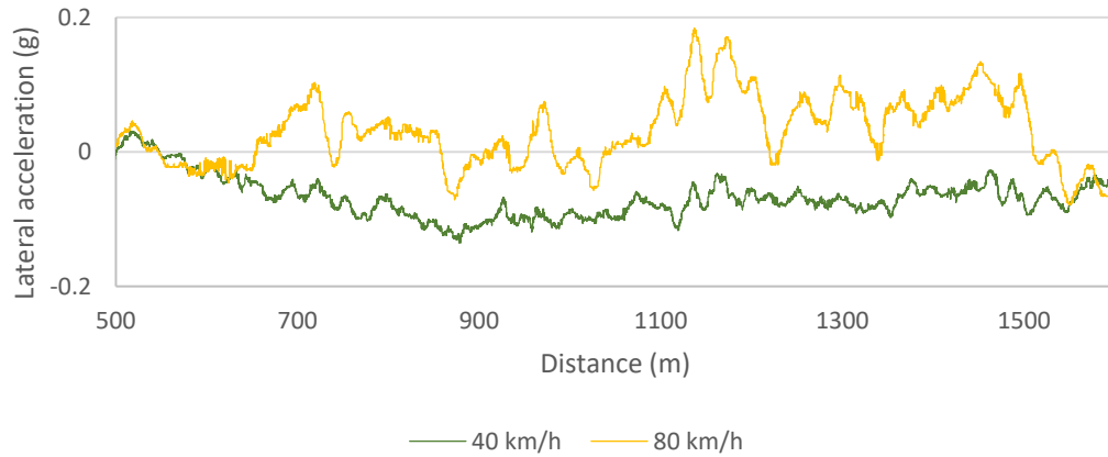
Figure 28 – Lateral acceleration on turn 1 & 2 (uncoupled 5-axle dog trailer combination)
