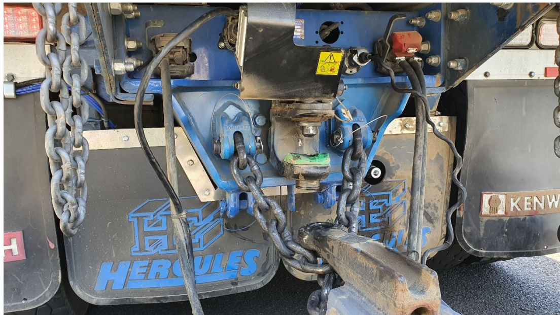
Figure 15 - Drawbar held by chains without coupling funnel
