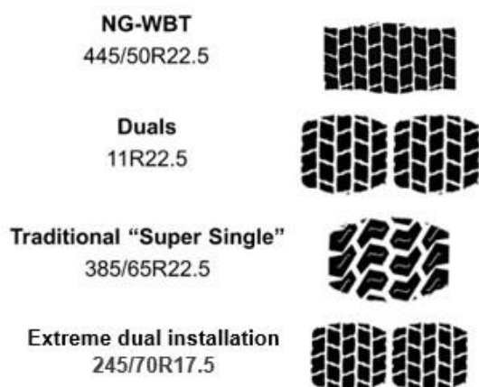
Figure 2.4 Illustrative comparison of shape and size of tyre footprints
