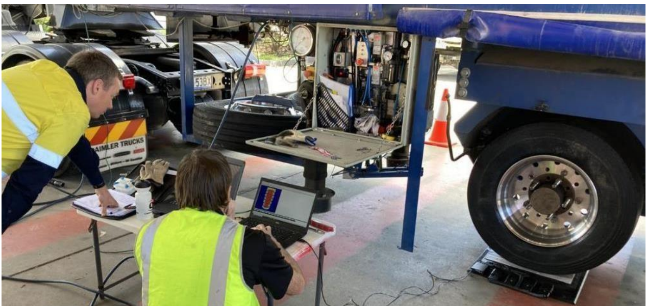
Figure 6.11 Field engineers from O'Brien Traffic and Goodyear recording tyre contact pressure distribution
