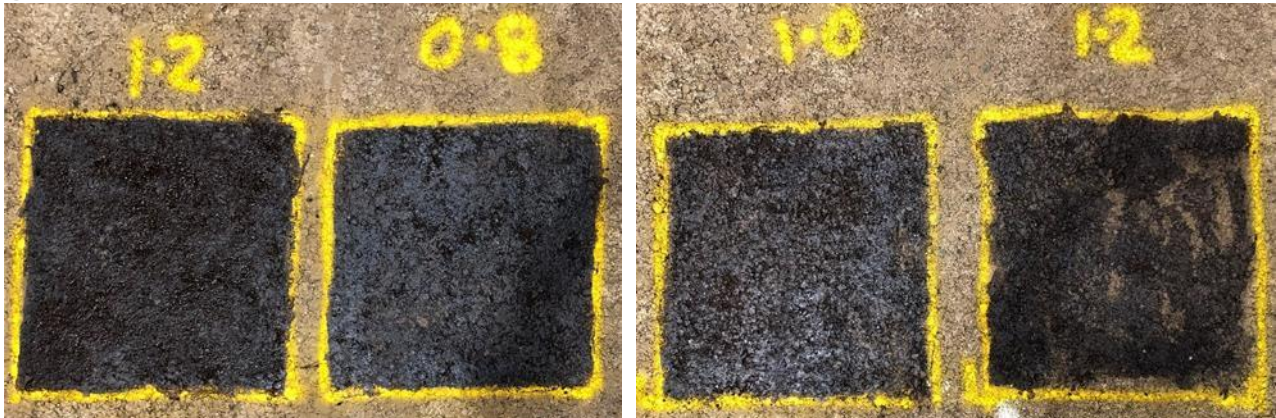
Figure 3.5 Primer trial patches
