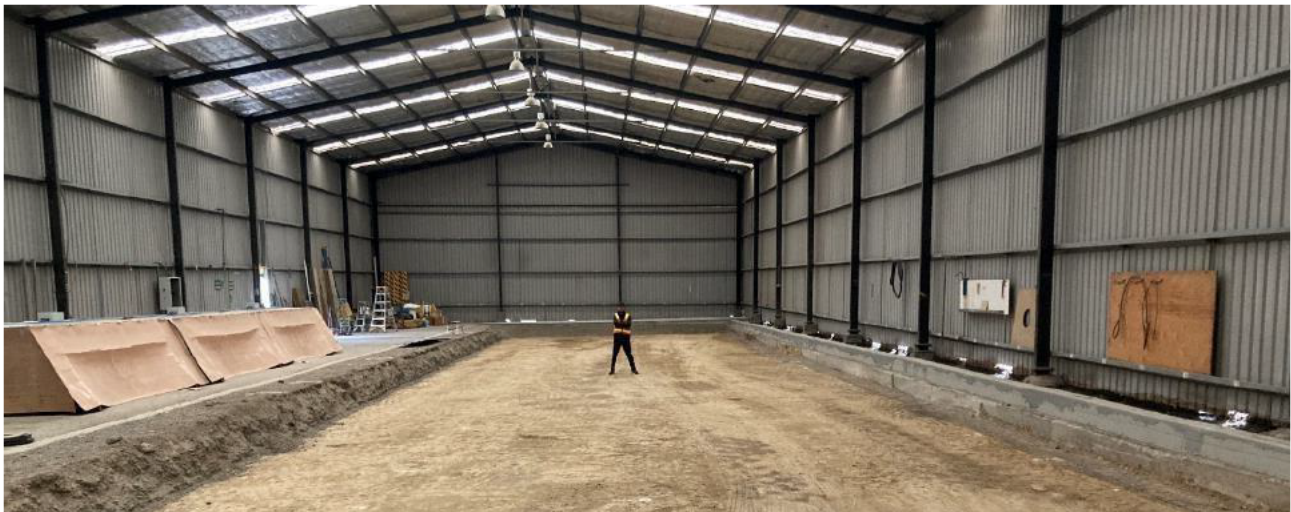
Figure 4.1 Test pavement subgrade and surrounding concrete walls
