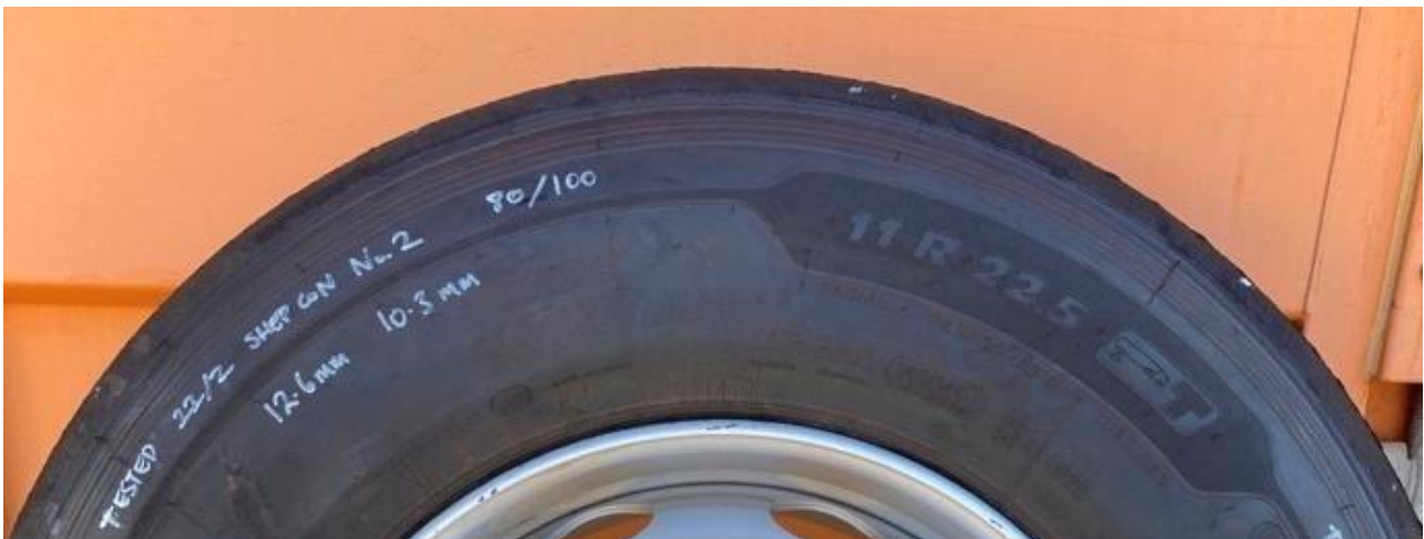
Figure 1.3 Tyre markings for an 11R22.5 truck tyre
