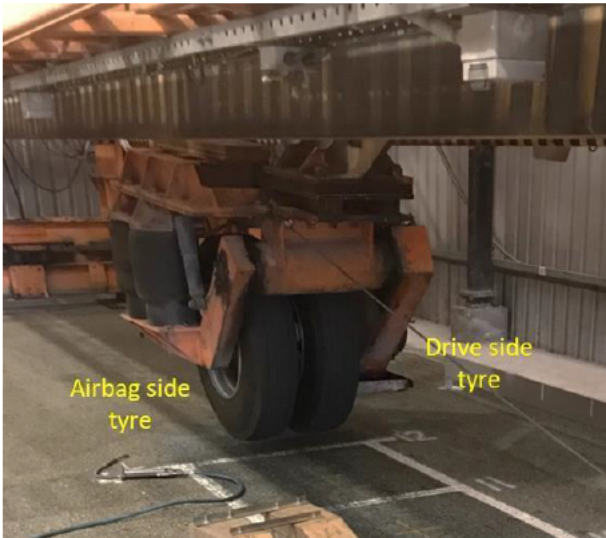
Figure 6.14 ALF configuration reference image for load distribution
