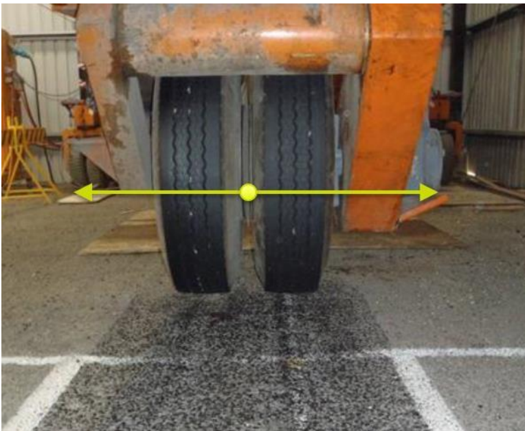
Figure 6.1 Transverse distribution of loading
