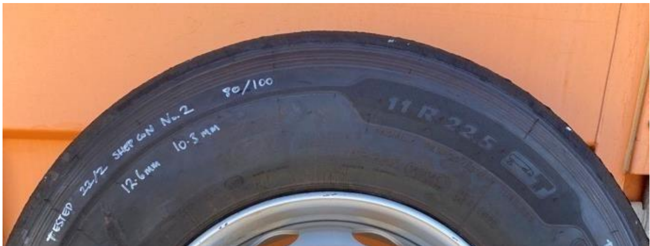
Figure 1.3 Tyre markings for an 11R22.5 truck tyre
