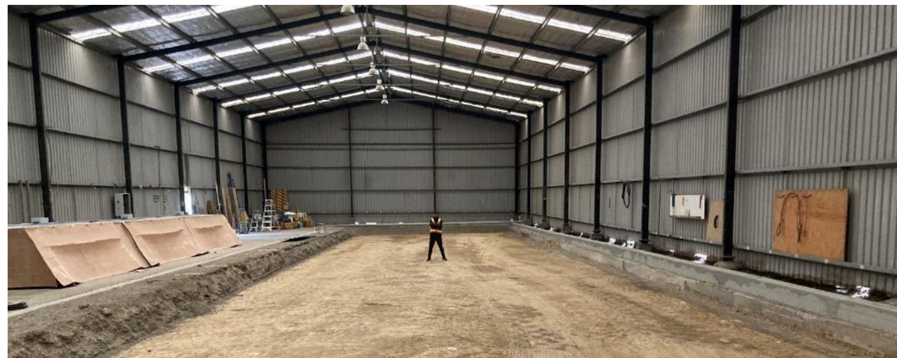
Figure 4.1 Test pavement subgrade and surrounding concrete walls
