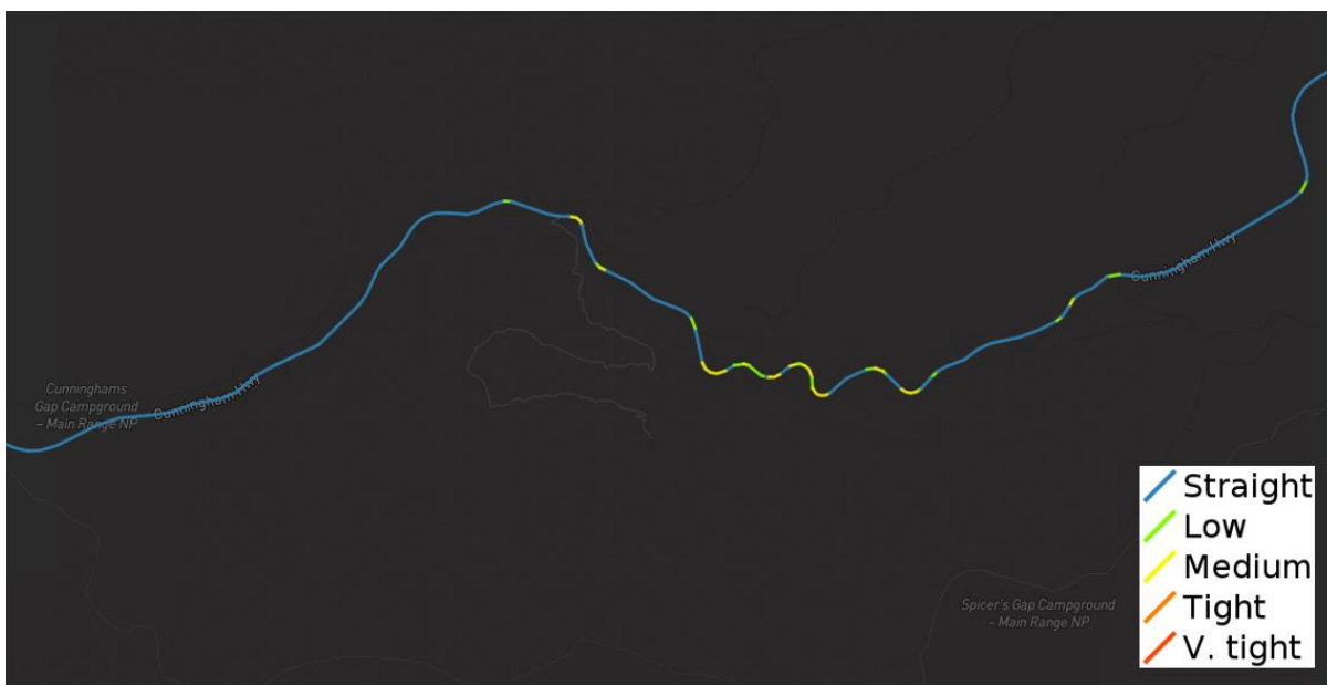
Figure 2.6: Road curvature (example 1)
