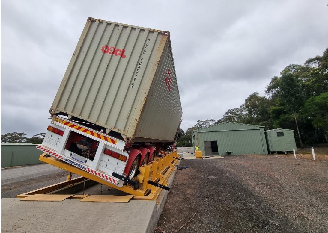
Figure 5: A photograph of an in-progress field test from the rear of the vehicle as it is tipped to the right
