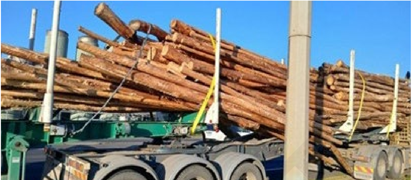
Figure 4.5. There was no headboard on the trailer.
