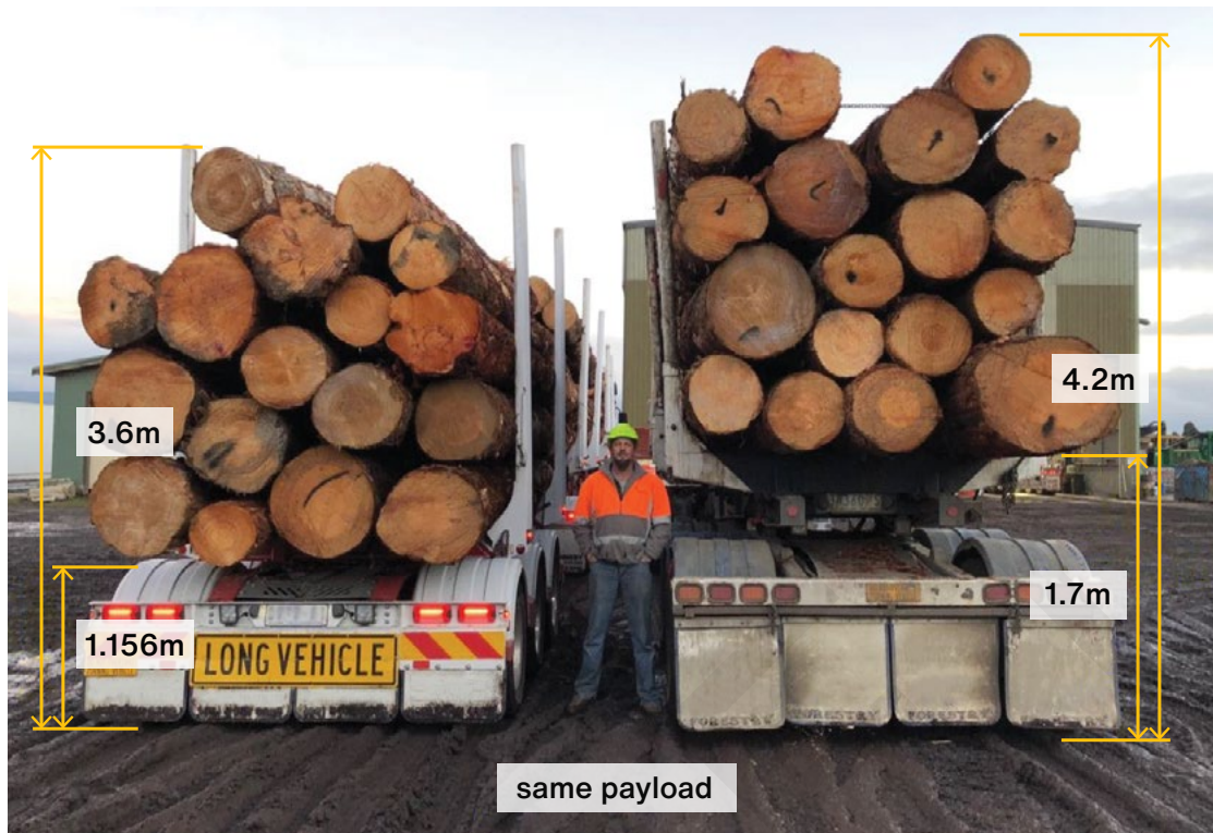
Figure 4.2. Step deck trailer with 19.5" wheels and low bolsters compared with flat deck with 22.5" wheels and high bolsters.
