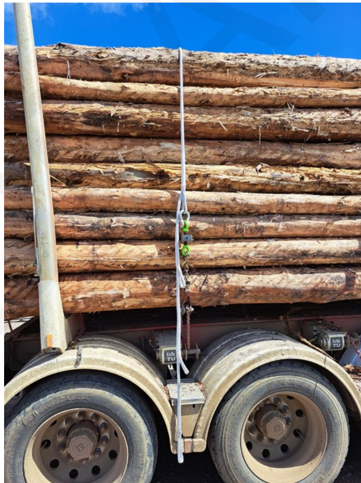
Figure A.3. A length of UHMWPE rope with eye splices at different lengths was used to position this load cell correctly.
