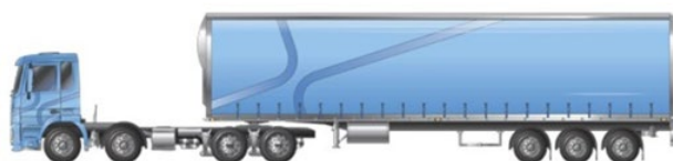
Figure 1: Twinsteer prime mover towing tri-axle semitrailer
