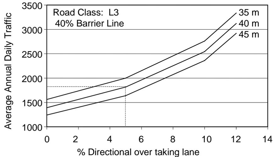
**Figure 1. An example of determining AADT for a target level of service for a given percentage directional overtaking lane**
