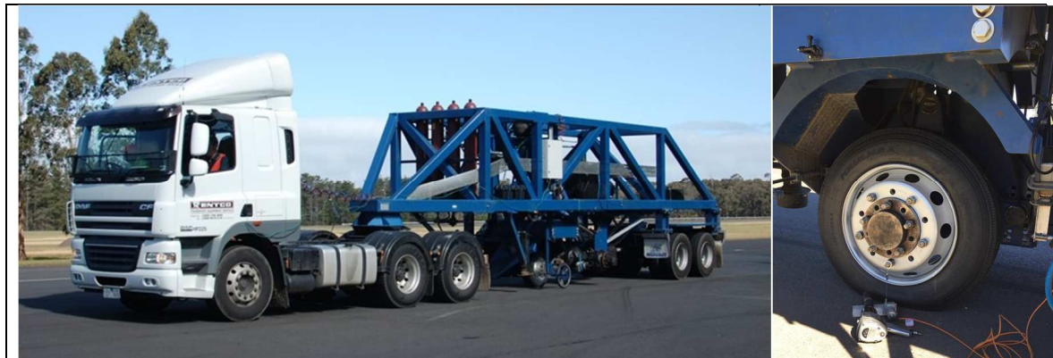
Figure 9. ARRB "over-the-road" tyre testing machine.
