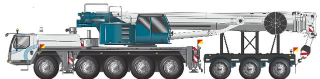
**Figure 6: Example of a typical Prescribed SPV that is a crane fitted with a support dolly**
