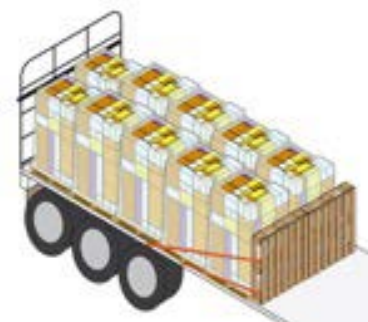
Figure 491 Pallet on end tied back
