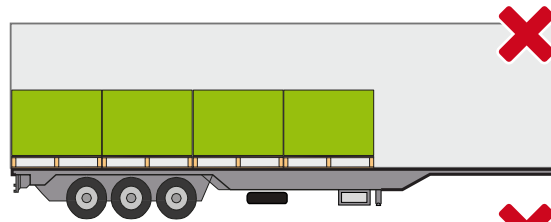
Figure 180 Gaps in contained load
