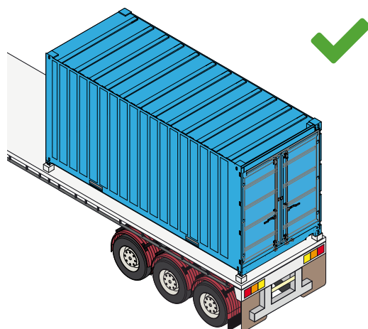
Figure 232 Loaded container with doors to the rear
