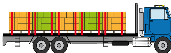
Figure 52 Pallets tied down
