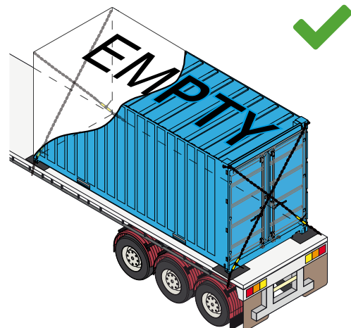
Figure 230 Empty container cross-chained
