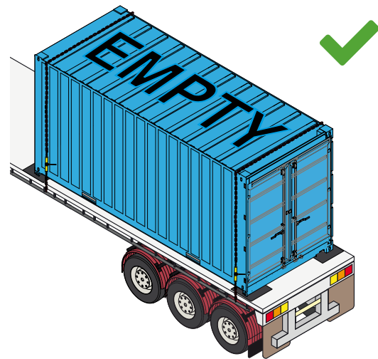
Figure 230 Empty container cross-chained
