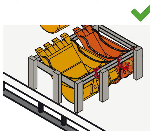
Figure 271 Restraint of auxiliary components
