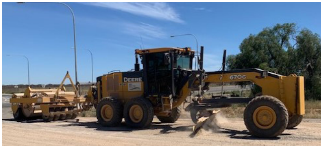
Figures 4 and 5: Motor grader towing one trailer or vehicle (maximum combination length 19m)
